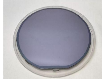
AlGaAs-on-Insulator following hybrid wafer bonding and substrate removal
